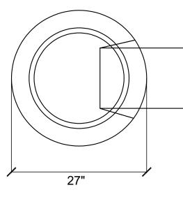
4", 6", 8",10" OR 12" PVC PIPE GROUT AS REQUIRED
