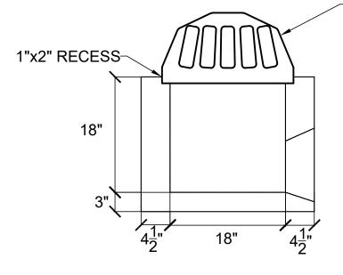
HMP R30 DOME GRATE OR R31 FLAT GRATE (NO FRAME REQUIRED)
