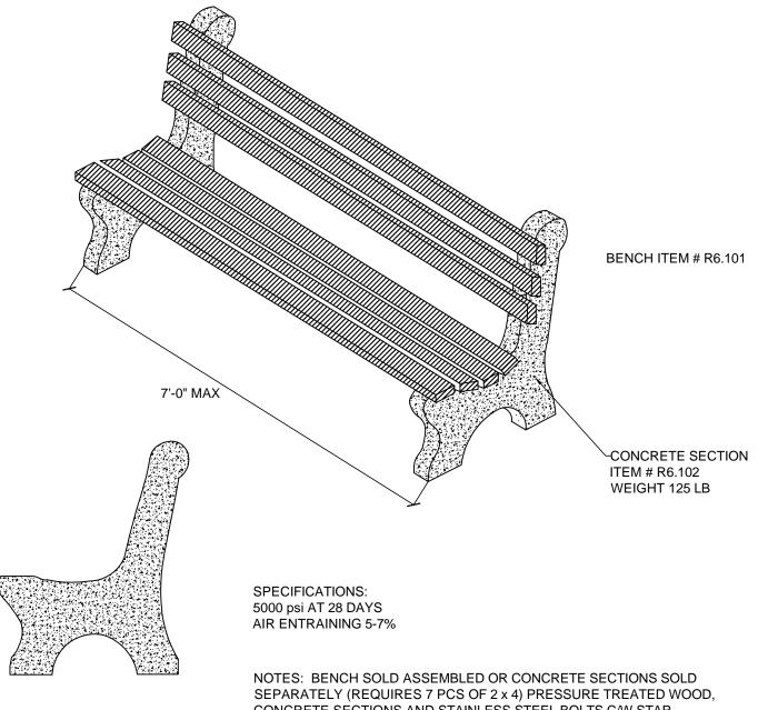
NOTES: BENCH SOLD ASSEMBLED OR CONCRETE SECTIONS SOLD SEPARATELY (REQUIRES 7 PCS OF 2 x 4) PRESSURE TREATED WOOD, CONCRETE SECTIONS AND STAINLESS STEEL BOLTS C/W STAR INSERT ALL COMBINE, TO PROVIDE AN ATTRACTIVE, MAINTENANCE FREE PRODUCT THAT WILL NOT RUST, CORRODE OR DETERIORATE THE SIMPLE DESIGN AND NATURE OF THE MATERIAL MAKE THIS PRODUCT A BEAUTIFUL ADDITION TO ANY SURROUNDING.
